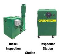
The Filter Inspection Station allows for the measurement of the filter condition before and after cleaning. To provide the best "real world" evaluation of the filter, a high power blower is used to draw air through the filter while the pressure drop accross the filter is measured.
