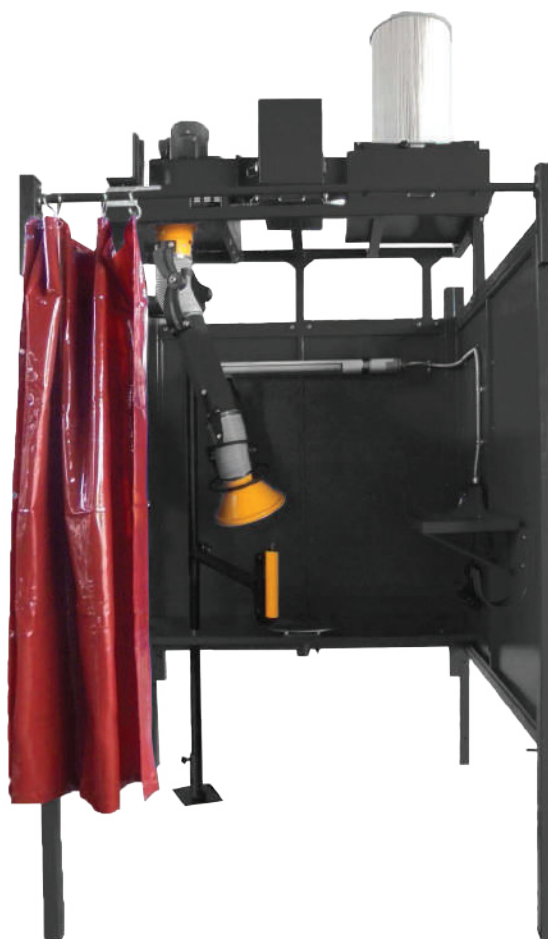
5'x5' 16ga. powder coated steel welding booth with rear shelf, standard curtain, CO2 bracket, c-clamp, lazy susan, light kit, top-mounted fume extraction system with 6" dia. fume arm
